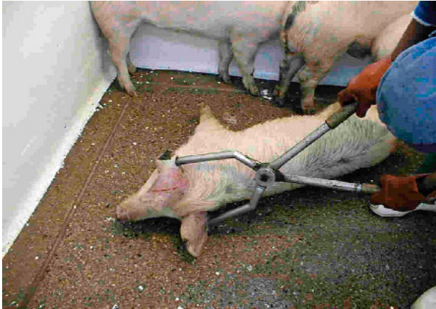
Fig. 58: Tongs for electrical stunning of pigs
