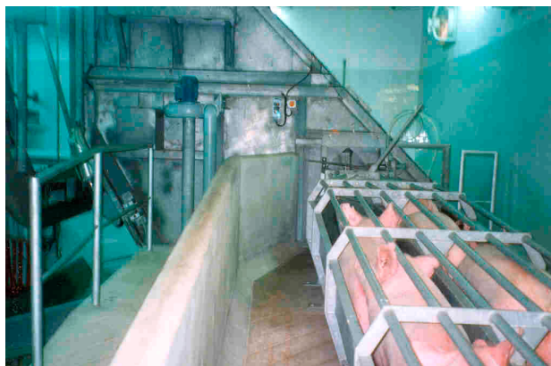
Fig. 65: Runway and entrance to a CO 2 -tunnel
