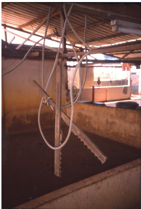
Fig. 70: Makeshift electric stunning tongs
