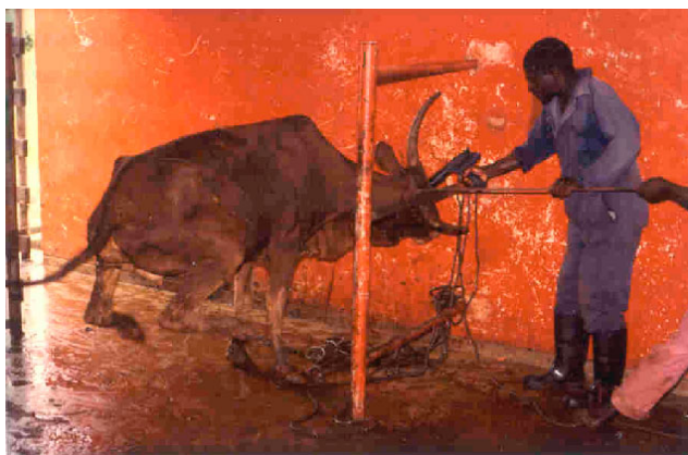
Fig. 46: Small-scale operation position of the pre-stunning operator behind protective steel bars
