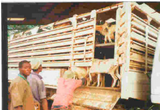
Fig.32: Double-deck truck for transporting sheep/goats
