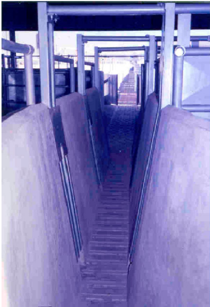
Fig. 24: Raceway for cattle from holding pens to stunning area
