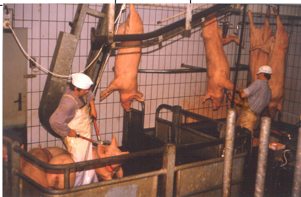
Fig. 77: Good arrangement for stunning and immediate bleeding of pigs at medium-sized
