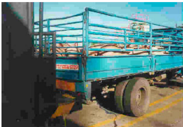
Fig.34: Well-ventilated truck for transporting pigs. Heat combined with hot sun would require a cover (roof) for the vehicle.
